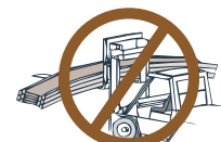
DO NOT lift I-Joists whilst they are lying flat. Excessive flapping may cause damage.
