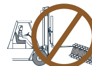
DO NOT lift or roll I-Joists by the top flange.
