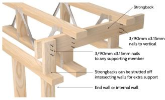
To ensure MultiStrut joists perform as intended it is critical that strongbacks are installed as per these details. Ensure strongbacks:
