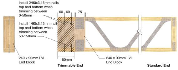
Note: Power driven nails must be used from top and bottom to secure end block after trimming. If trim is 120mm+ then nailing is not required
