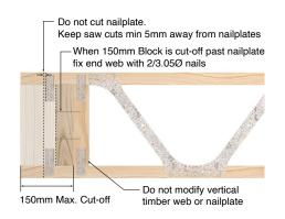
Note: If remaining block is less than 25mm the block piece is not required.
