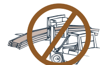
DO NOT lift I-Beams whilst they are lying flat. Excessive flapping may cause damage.
