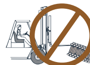
DO NOT lift or roll I-Beams by the top flange.
