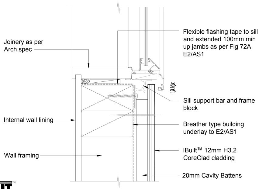
IBuilt<sup>™</sup> CoreClad Ply Cladding is to be installed as per the requirements of Clause E2/AS1 Section 9.8
