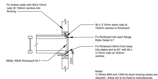
specifications in addition to the fixing shown above. 2) Other wall fixings to NZS 3604 requirements.
