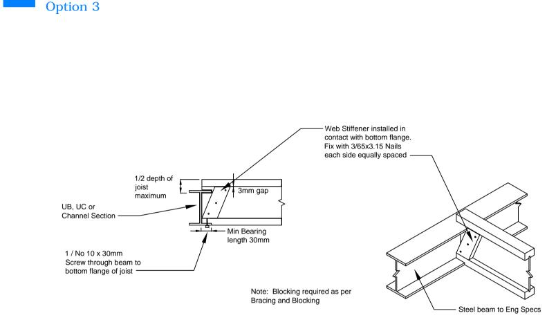
Joist Connection to Steel Beam
