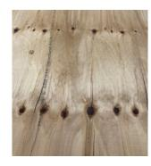
DD - D quality to both faces. Non-appearance grade that contains knots less than 70mm and other unfilled defects. This is the most basic structural panel suited to nonvisual structural applications.
