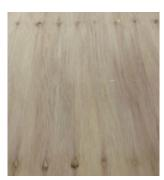
CD - C quality front/D rear face. Sound knots less than 50mm and open defects on the face are filled and sanded. Applications could include substrates for membrane systems, formwork, flooring, roofing and bracing.
